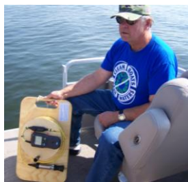
Tom Stram getting ready to use the temperature recording device. We record at 5'0" intervals to a depth of 80 feet.
