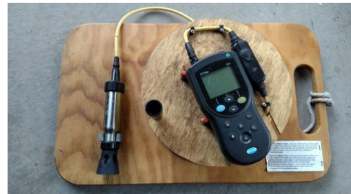
The oximeter is used for water temperature & dissolved oxygen readings. We test to 80 feet on Connors Lake and 35 feet on LOP.
