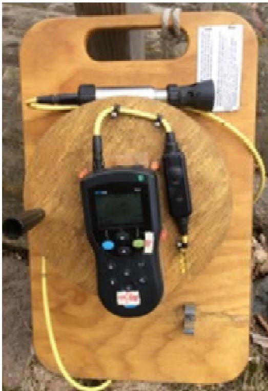
A piece of equipment that our lake association purchased, which greatly reduced the collection time and improved the accuracy of our data, was a HQD digital meter from the Hach Company. With this instrument, we can sample dissolved oxygen and temperature simultaneously. We do this at the lake’s surface and at five-foot intervals. Samples are always taken in the deepest spot in the lake (Connors is 80 feet and LOP 35 feet).
